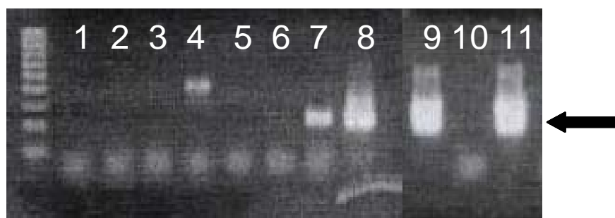
Figure 3. PCR products of nested amplification with COI primers. Lane 1: fragment identified as "not Lepidoptera". Lanes 2, 3, 4, 5: bat droppings. Lanes 6,7: droppings with C. suppressalis antenna and tarso added. Lanes 8,9, 11: C. suppressalis . Lane 10: Blank sample, without any DNA. The white arrow show the 99bp and the 202bp long positive bands.
